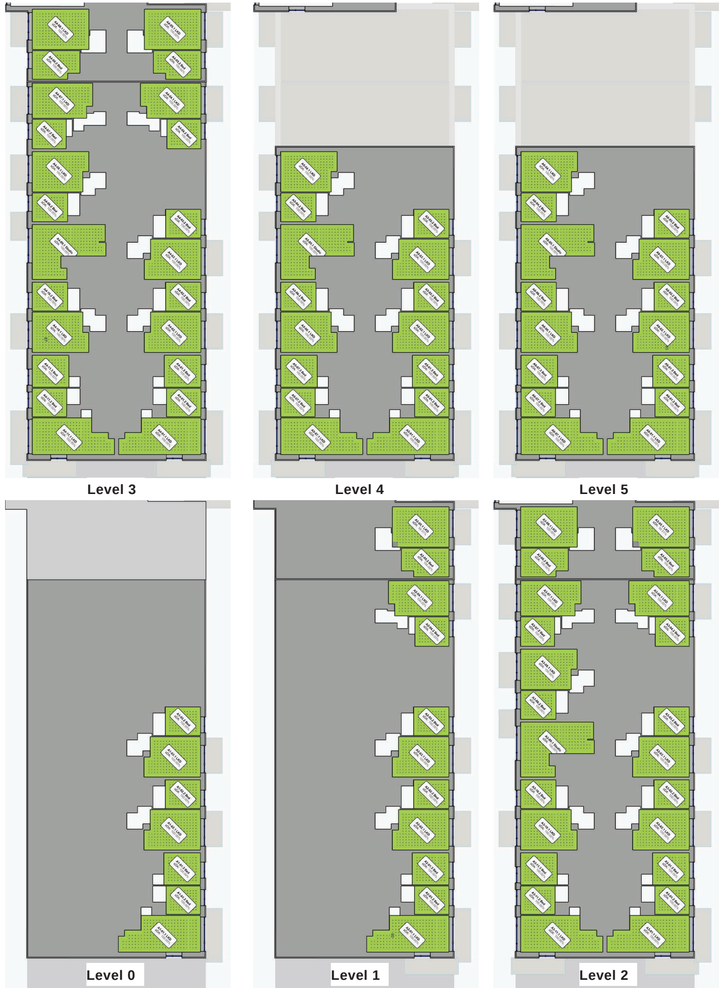
Figure 28: Block A - Floor plans indicating Daylight Provision to BS EN17037:2021+A1 Table NA.1
